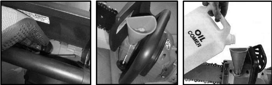
Figure 7 – Oil filling for chain lubrication.
