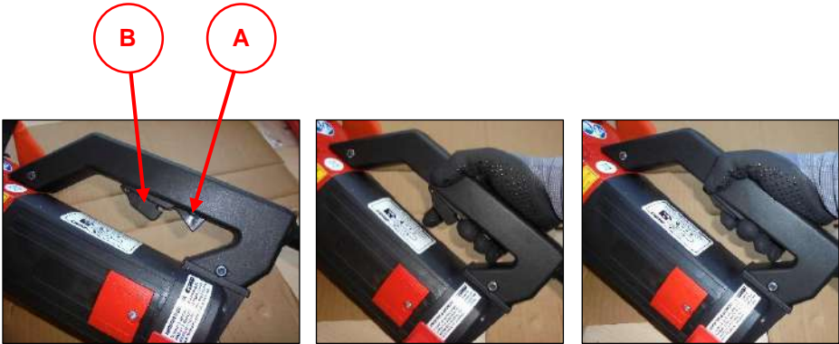
Figure 12 – Push the safety block switch (A) and then the Start button (B).
