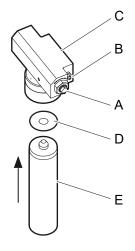
The pump unit (C) must always be sealed to prevent the ingestion of water and dust.
