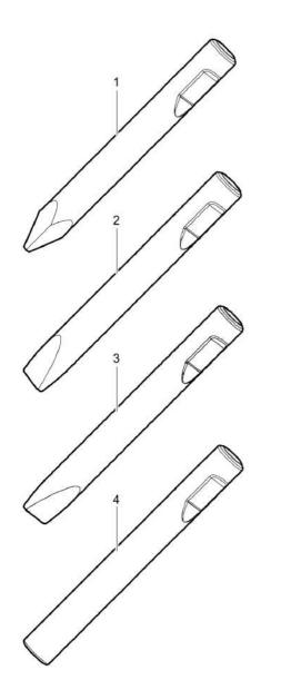
Ø=140 mm, L=620 mm, L\_{\tau}=1150 mm, Wt=120.6 kg Ø=5.51 inch, L=24 inch, L\_{\tau}=45.28, Wt=265.9 lb
