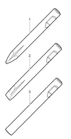
Ø=140 mm, L=670 mm, L\_{\tau}=1200 mm, Wt=125.5 kg Ø=5.51 inch, L=26 inch, L\_{\tau}=47.24, Wt=276.7 lb
