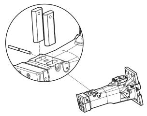
NOTICE The lock buffer in the tool retainer lock is made of plastic and can melt when operating in a hot environment. If this occurs, change the standard lock pin. Find optional spring pin in the spare parts list.
