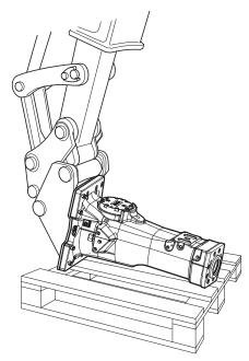
The pressure inlet on the hydraulic breaker is on the left side when you are facing the accumulator. If the pressure hose is on the other side of the boom you can cross the hoses or turn the hydraulic breaker.
