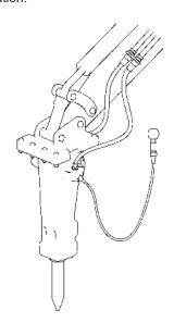
Position the hydraulic breaker vertically towards solid bedrock or similar to adjust the pressure using a pressure gauge.
