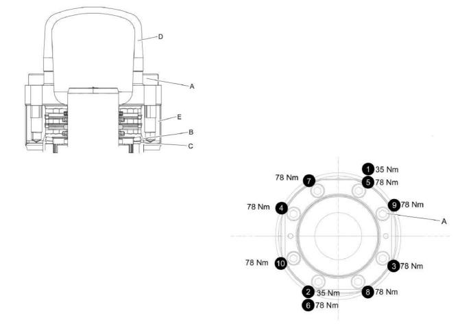
1. Make sure the spring plate (B) and spacer (C) are centered before mounting the back head (D).
